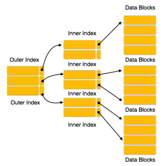
Multi-level Index helps in breaking down the index into several smaller indices in order to make the outermost level so small that it can be saved in a single disk block, which can easily be accommodated anywhere in the main memory.
